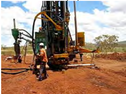
Reverse Circulation (RC) rig, outside Newman, Western Australia
