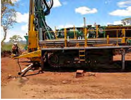
Track mounted Reverse Circulation rig (side view).
